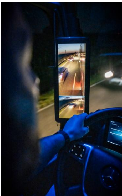
Figure 3: Nighttime View of the MirrorCam Left Display
