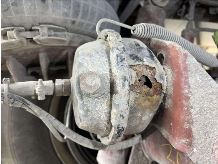
Figure 2: Air leakage occurring in the brake cylinder (M. M. Sanchez, 2026)
