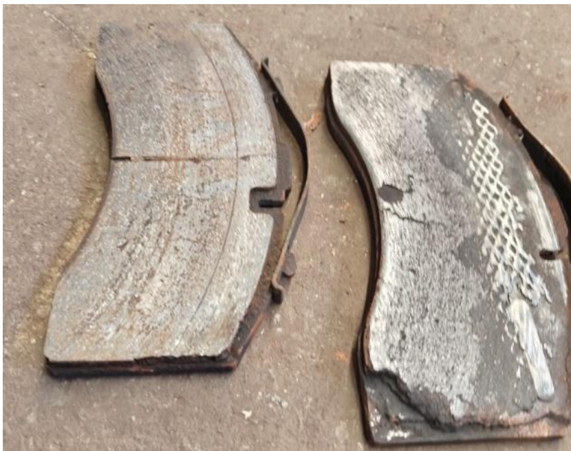
Figure 4: Severely worn brake linings (M. M. Sanchez, 2026)
