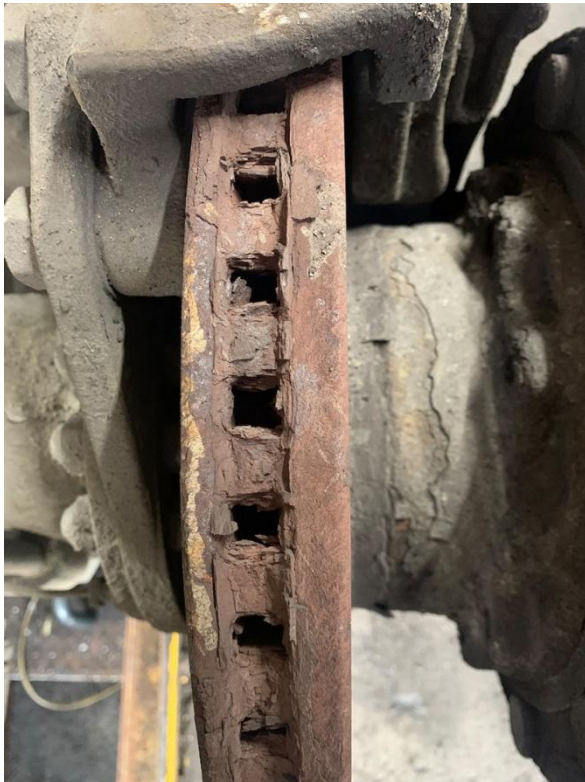
Figure 7: Severely worn brake disc (M. M. Sanchez, 2026)
