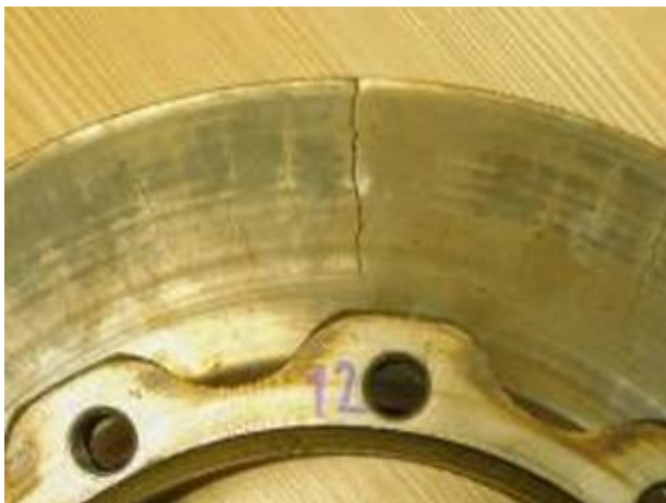
Figure 5: Crack formed on a brake disc (Hasanlu et al., 2025)
