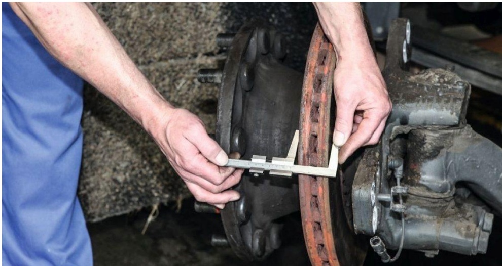
Figure 6: Inspection of brake discs (ZF Aftermarket, 2026)
